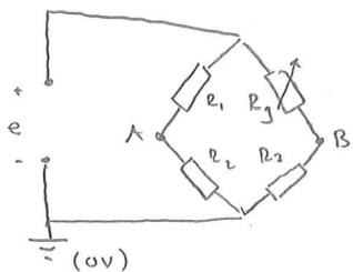
$$e_A = \frac{R_2}{R_1 + R_2} e$$
