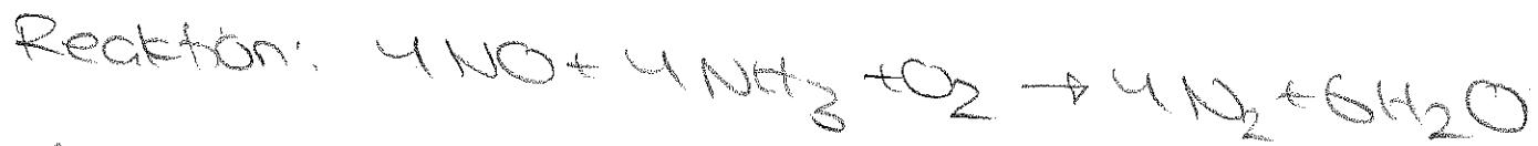
Katalysator, ex: 1,5% V<sub>2</sub>O<sub>5</sub> + 9% WO<sub>3</sub> on TiO<sub>2</sub>
